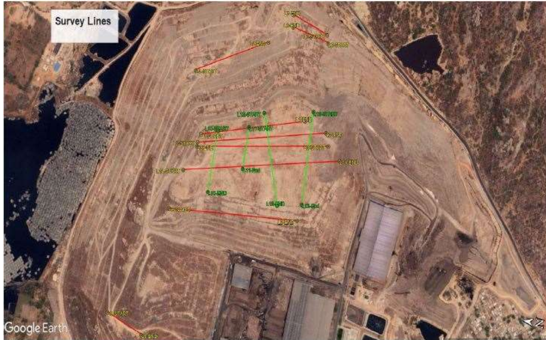
Plate 5.1 The Google Earth map exhibiting the actual stretches of the MASW and ERT investigations
