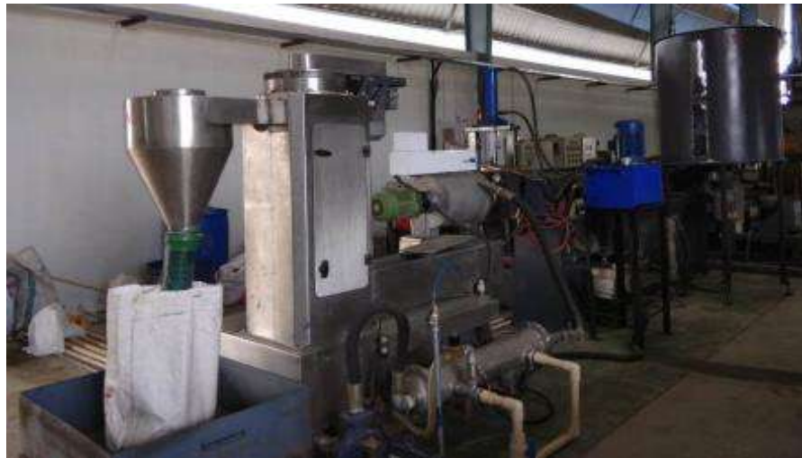
Extruder - Recycled Granules Making Process
