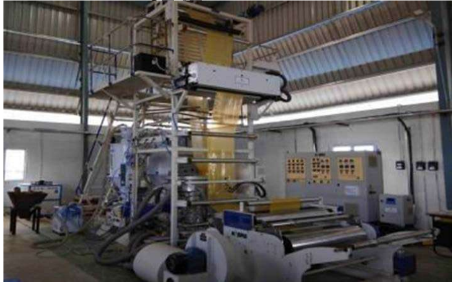
Film molding for production of bags for waste disposal
